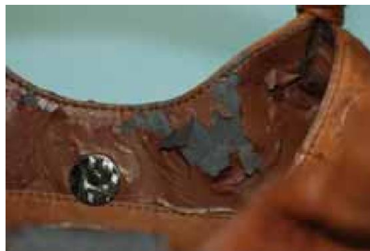
Figure 11 Case Study of Surface Peeling of Synthetic
