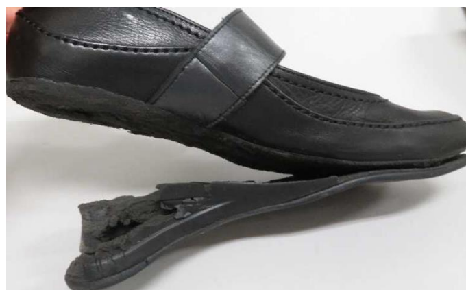
Figure 6 Case Study of Polyurethane Outsole Broken
